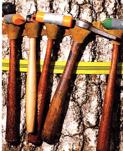
The mallets Holand uses for the repoussé work on his weathervanes have custom-made tips for specific uses and projects.
